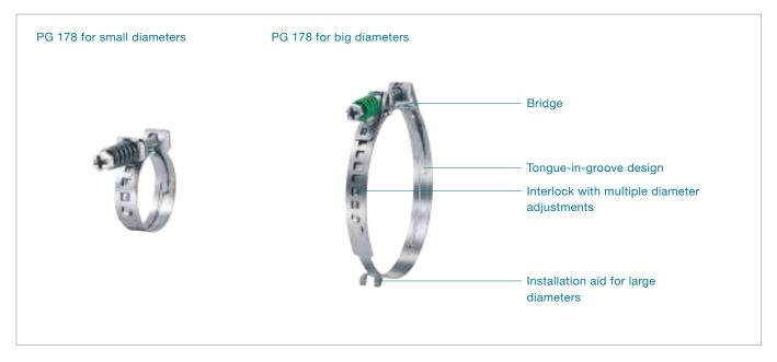
Choice of engagement positions: clamp can be adjusted to several different nominal diameters Narrow Band: concentrated transmission of clamping force, complies with SAE J1508 Type SSPC 360° Stepless®: uniform compression, or uniform surface pressure. Burr-free strip edges: reduced risk of damage to the part being clamped Self-tensioning: compensates for thermal cycle diameter changes
