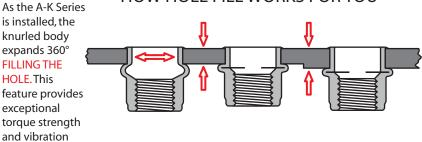
The installation tool then continues to install the insert forming a backside flange even in multiple or variable thickness materials WITHOUT ADJUSTMENT.
