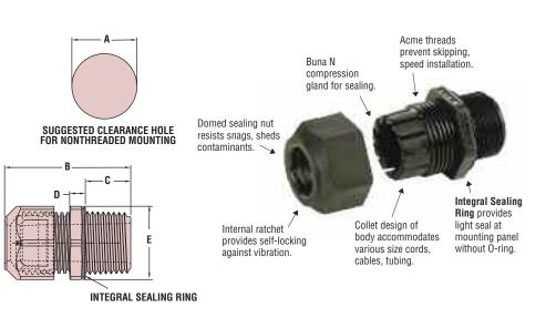
Material Nylon 6/6 Non-halogenated w/Buna N Sealing Gland Listed under Underwriters' Laboratories File E51579 Certifications **Recognized under the Component Program of Underwriters**' Laboratories File E51579 Ð Certified by Canadian Standard Association File 93876C Approved for NEMA 4, 4X, 6 and 6P Applications Flammability Rating 94V-0 **Temperature Range** Static -40°F (-40°C) to 239°F (115°C) Dynamic -4°F (-20°C) to 212°F (100°C) **IP** Rating IP 68 (70 PSI, 5 BAR)
